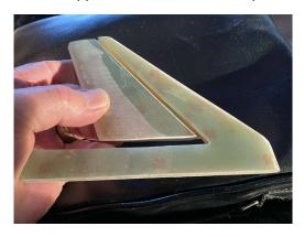
And here is the view of the tip. You can see I made it by gluing 3 sheets together so the center sheet – which is thin and bendable – acts as a hinge. After laminating them I sanded the back edge to a thin tip to act like solid fins.
