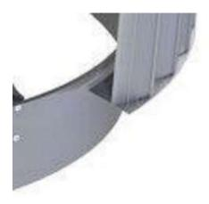
That gap allows the top to rotate. In order for this design to be complete this gap must be closed. You can see that there is a metal plate at the bottom to which the blades attach. I imagined that if the entire assembly of blades were moved up or down then another plate could be attached below this plate so if the top were lowered the gap would be closed.
